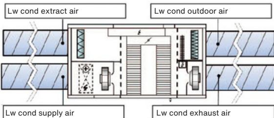
Curves are built on outdoor air (Static Pressure) with all round spigots connected to the ducts (D configuration for NF EN 13141-4 concerned)
